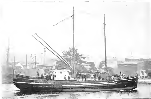
Halibut schooner Scandia, equipped with 2-cylinder, 160 brake horsepower Bolinder engines.
